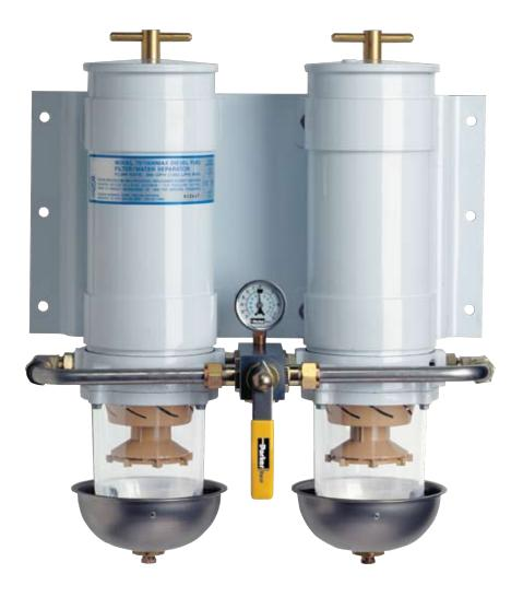
A single valve on all of the double manifold MAX models isolates one filter/separator for service while the other keeps operating. This way, you keep running while draining contaminants from the collection bowl or while changing filters.
