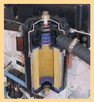
Cummins QSM11 marine engine with CCV cutaway
