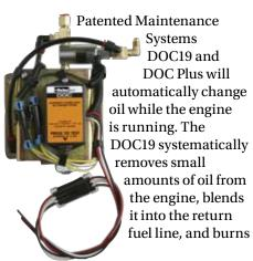
it as fuel—in a simple, efficient closed loop system to keep your vehicle out of the maintenance shop and on the job. The DOC Plus incorporates Racor's proven gravity-based Never Lo oil replenishing system to continuously replace the oil withdrawn from the engine and burned by the action of the DOC for the ultimate in hands off oil maintenance. Reduced downtime for engine maintenance means quick payback.
